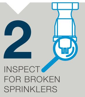
While your center pivot is running with water, inspect all sprinklers and look for plugged or broken sprinklers, uniform water patterns, and leaking sprinklers or pressure regulators.
